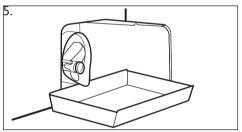
Pull out the emergency emptying cap from the filter cover, using pliers.
